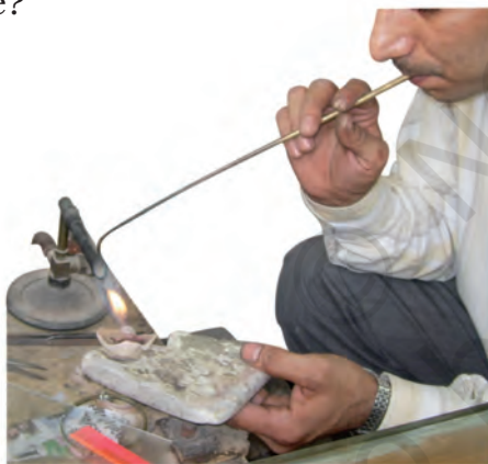
Fig. 6.14 : Goldsmith blowing through a metallic pipe
